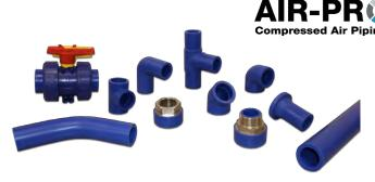
SDR 7.4, 230psi: 20 - 110mm (1/2" - 4") **SDR 11, 150psi:** 160 - 315mm (6" - 12") Welding: Butt, socket, electrofusion
